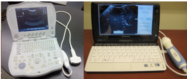
Figure 1: Comparison of GE LOGIQBook (left) and our simplified device (right)
